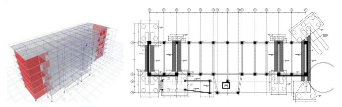
Image 3. Model with shear walls as SFRS
