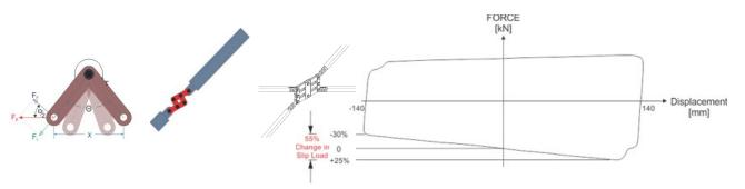
Image 11 Variation in force in rotational mechanisms
